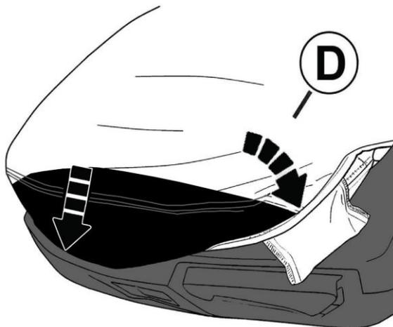
Tuck side edge of seat cover into the plastic trim of the seat, starting at the front and working your way to the back.
