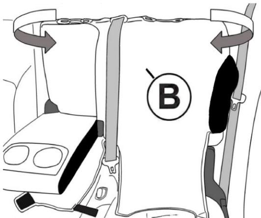
Wrap the top section of the seat cover around the top corners of the seat. Align the hole for the seat-belt and re-fasten the Velcro®. Position the bottom of the seat cover as shown.
