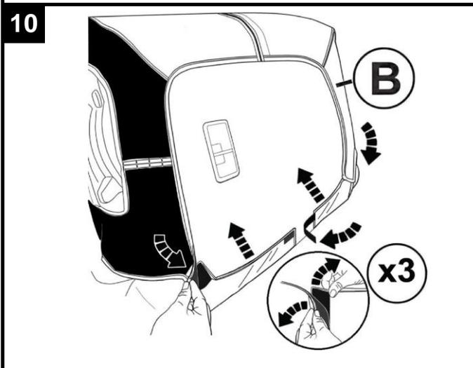
Fasten 3 Velcro® sections at the back of the seat. Ensure that the seat cover holes align to the headrest post holes.
