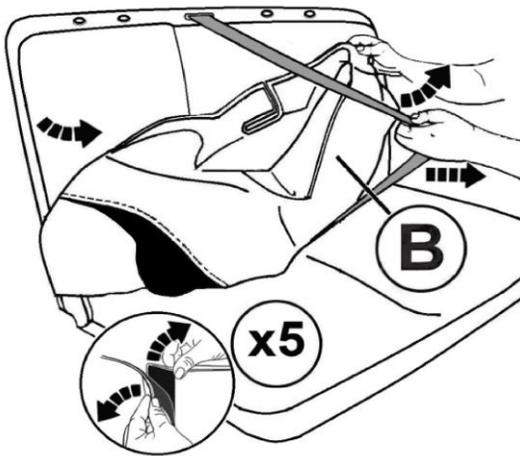
Unfasten all Velcro® connections in **B** (x5) and thread seat cover under seat belt. Open center armrest.
