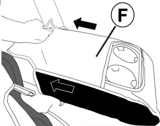
Pull **F** over center armrest. Ensure hole aligns with center armrest cup holders.
