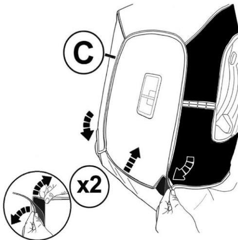
Fasten 2 Velcro® sections at the back of the seat. Ensure that the seat cover holes align to the headrest post holes.
