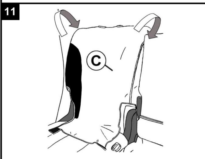
Unfasten all Velcro® connections in **C**. Wrap the top section around the top corners of the seat while tucking the seat cover between the seats. Align the holes for the headrest posts. Position the bottom of the seat cover as shown.
