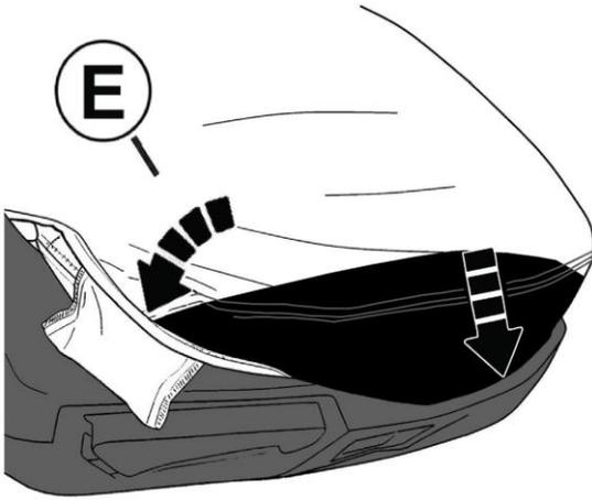
Tuck side edge of seat cover into the plastic trim of the seat, starting at the front and working your way to the back.
