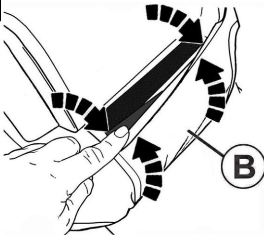
Fold armrest up and fasten Velcro® edges tightly.
