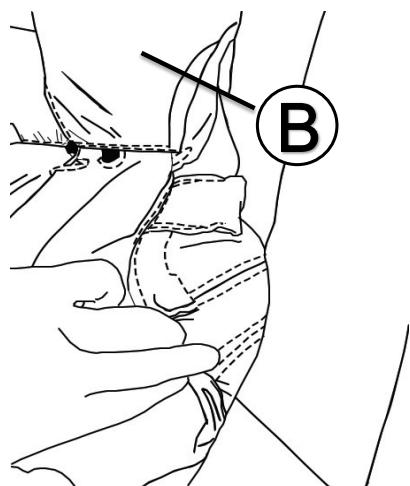
Tuck all covered inserts on side edge of the seat cover into the plastic trim of the seat. Starting at the front and working your way back. Repeat for the other side.
