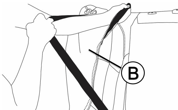
Move center seat belt to the side, and align hole at the top of the seat as shown.
