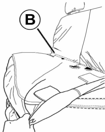
Wrap seat cover around the front corners of the seat. Repeat for the other side. Tuck center padded insert between seat and floor.
