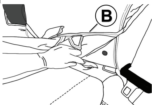
Position the seat cover bottom and tuck bottom center padded inserts between the seat back and seating surface.
