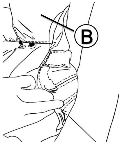
Tuck side edge of the seat cover into the plastic trim of the seat. Starting at the front and working your way back. Repeat for the other side.
