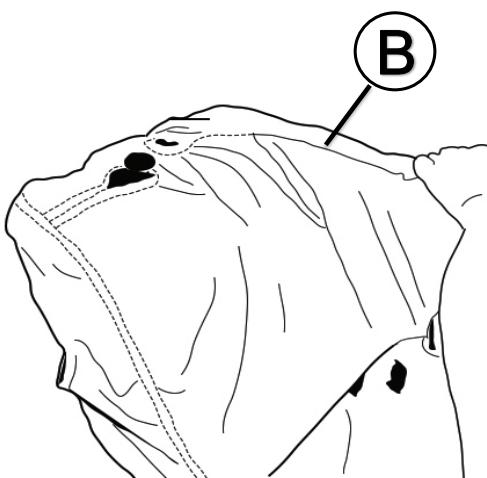
Align all holes at the top of the seat as shown.
