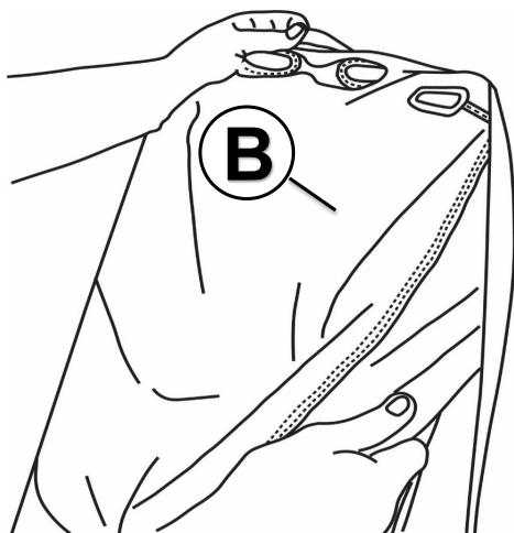
Wrap the cover around and over the top part of the driver's seat. Align all holes at the top of the seat as shown.
