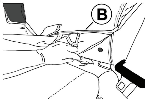
Position the seat cover bottom and tuck bottom center between the seat back and seating surface.
