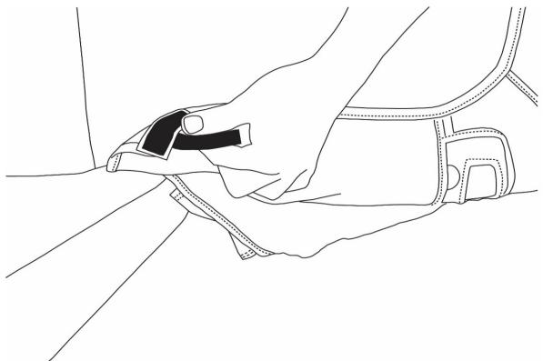
Fold seat down and fasten Velcro® section at the back of the seat.
