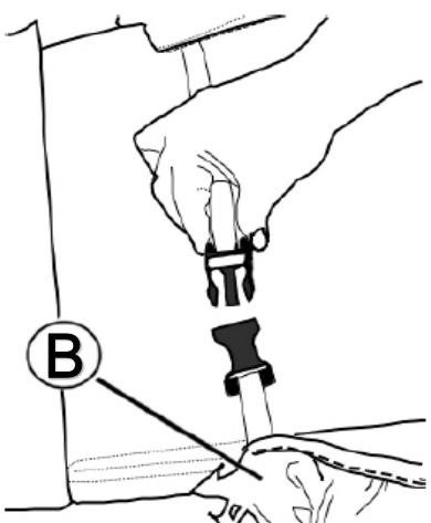
Fold seat down and connect buckle then tighten the straps.
