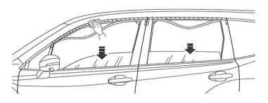
Install clips (5) onto side window deflectors as shown.
