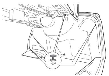
Ensure the claws from the Rear Trunk Trim Panel are properly aligned before fully engaging. Adjust weatherstripping if necessary.
