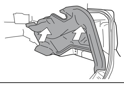
Re-install the five clips holding the Right Side Trunk Trim Panel. Repeat for the left side.
