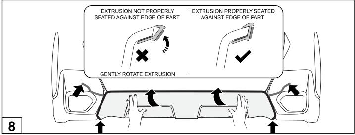
Re-inspect gasket to ensure that no areas are "rolled under" prior to installation.
