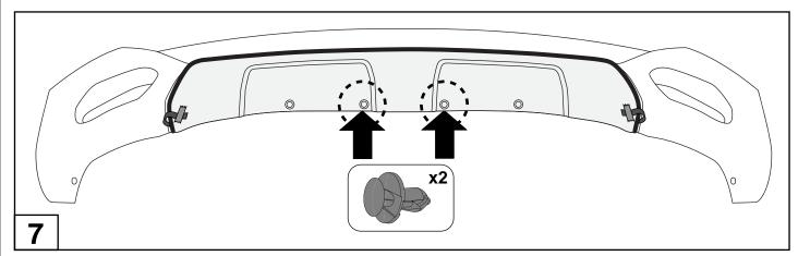
Install (2) provided retainer plugs in the inner available holes in Bumper Under Guard.
