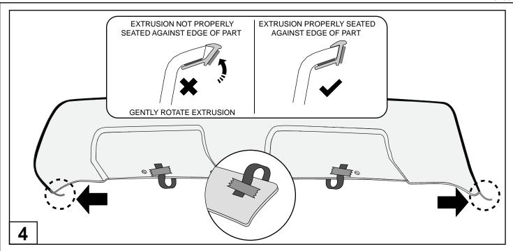
Inspect gasket conformity to Bumper Under Guard prior to installation. Rub gasket if needed, to ensure it is not rolled away from edge of Bumper Under Guard. Peel back approx. 50mm / 2" of tape liner at each end of the part and fold at 45 degrees to part. Tape peeled back section of tape liner to outside surface of the Bumper Under Guard using masking tape.
