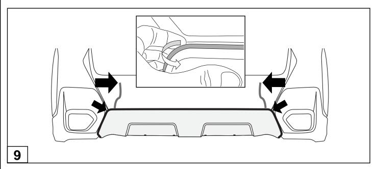
Rotate rubber gasket outwards while applying light forward mounting pressure to enable gasket to lay flat on bumper, carefully remove additional liner from the corner radius, pulling the liner in the direction in which it is being removed, until the corner is passed to be on the final long straight edge. Repeat for the opposite side. Apply forward pressure to adhere the corners of the Bumper Under Guard to the bumper surface.
