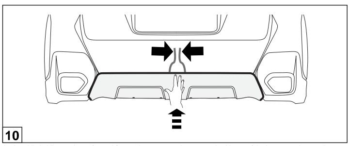
Again, while holding moderate forward / upward pressure on the center raised bump of the bumper under guard, ensure that the rubber is still properly aligned with the feature line in the rear bumper. Then begin pulling each remaining tape liner, one side at a time, to meet in the center of the part and ultimately removed completely.
