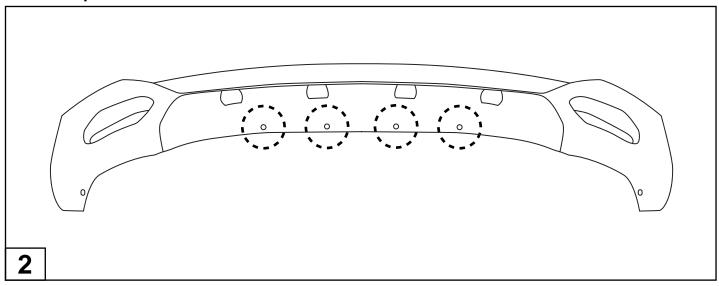
Identify (4) holes in factory bumper that will align with holes in Bumper Under Guard.
