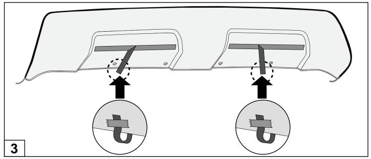
Peel back enough tape liner at each end, to go past the first (outer) mounting hole, then fold at 45 degrees to part. Tape peeled back section of tape liner to outside surface of the Bumper Under Guard using masking tape.
