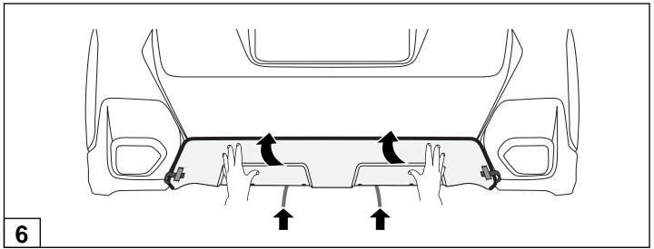
Peel remaining tape liner from center taped sections of Bumper Under Guard, then push up and forward in a rotating motion to ensure these taped sections get good contact with rear bumper.
