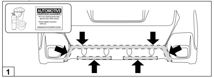
Make sure that all installation surfaces are clean, free of dirt, grease and debris using soap and water solution. Clean the indicated (shaded) tape adhesion area with the alcohol wipe (provided).
