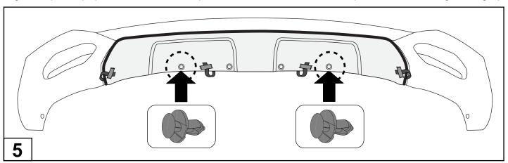
Hold Bumper Under Guard in position of best fit and in line with factory holes. Install (2) provided retainer plugs in the outer available holes in Bumper Under Guard.
