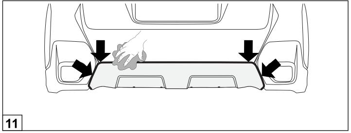
Apply moderate palm pressure across the entire top and side leading edges where the tape is contacting the bumper. Use a dry and clean microfiber towel to continue rubbing pressure along these same areas approx. 5 times in a consistent direction from one end of the Bumper Under Guard to the other, to ensure proper tape adhesion and compression is achieved.
