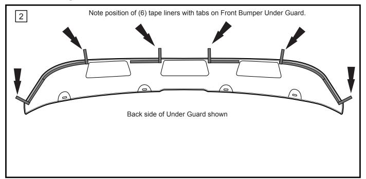
Fold the tape liner tabs over the edge and use masking tape to hold the tabs to the front outside surface of the Under Guard so that the liner does not fall back under the part during installation.
