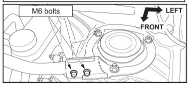
(7) After installing, Use gauge to check the clearance between the bar and the vehicle. When clearance is not enough, loosen the flange nut.
