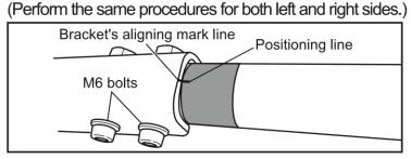
extension of the aligning mark line of the bracket.
