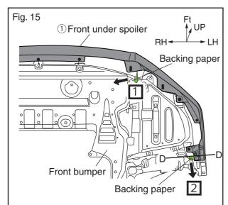
(7) Remove the backing paper from the double-sided tape attached on the front under spoiler ① in the directions shown by the arrows in the order of 1 and 2 shown in the figure, and firmly press the double-sided tape portions with a force that can move the vehicle slightly. (Fig. 15)
