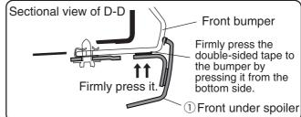
**△** CAUTION When removing the backing paper, be careful not to allow the backing paper to break at midpoint.
