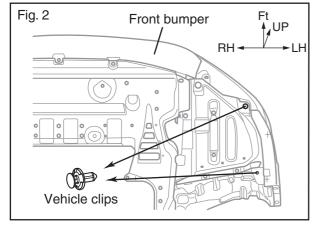
The removed vehicle clips will not be reused.
