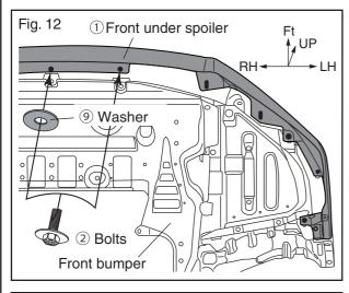
(4) Temporarily fix the front under spoiler ① with the bolts ②. For the center portion, insert the washer
