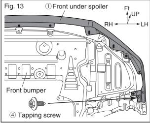
(5) Temporarily fix the front under spoiler ① with the tapping screw ④. (Fig. 13)(1 location each on RH and LH, 2 locations in total)
