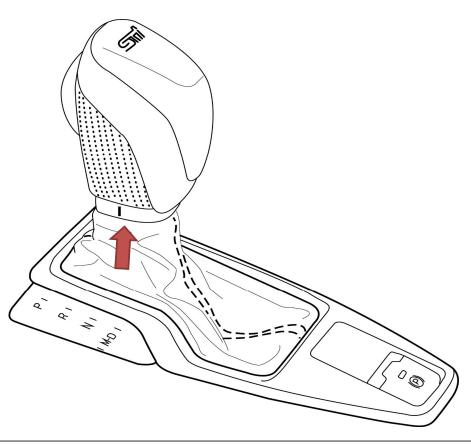
STEP 6: Depress brake pedal. Confirm that the shift knob is firmly installed and that the button can be fully depressed. Make sure the shift knob is properly installed before operating the vehicle. Turn on ignition, depress and hold brake pedal, confirm shift lever cannot shift out of "P" without depressing button. Confirm shift lever function by checking engagement into Reverse and MD modes.
