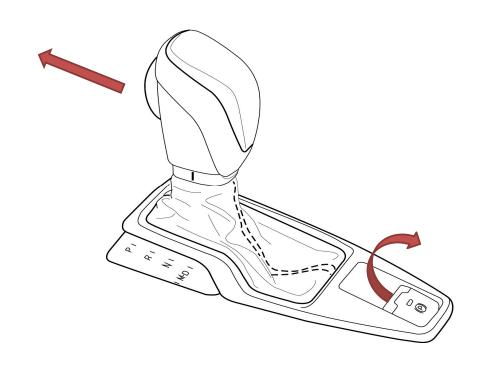
STEP 2: Use plastic trim removal tool to pry and push down on the factory cover grip.
