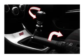
Disconnect the negative cable from battery and make sure parking brake is applied firmly. Remove the original shift knob by turning counter-clockwise.
