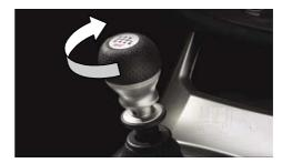
Remove any dust on the stalk with a clean brush and screw the Shift Knob onto the stalk until tight.
