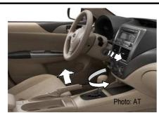
Disconnect the negative cable from battery and make sure parking brake is applied firmly. Unscrew and remove existing shift knob.
