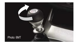
Remove any dust on the stalk with a clean brush and screw the Shift Knob onto the stalk until tight.
