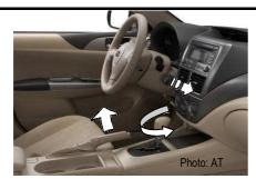
Disconnect the negative cable from battery and make sure parking brake is applied firmly. Gently pull shift boot down from stock shift knob. Remove original shift knob by turning counter-clockwise.
