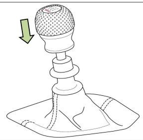
STEP 5: Turn STI Leather Shift Knob clockwise until tight. Do not overtighten. If needed, turn the knob slightly counter-clockwise until the STI logo is in the correct orientation.
