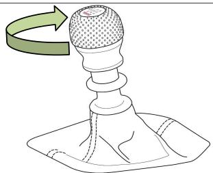
STEP 6: Check the operation of the shift lever by moving it through each gear including reverse. Installation Complete.
