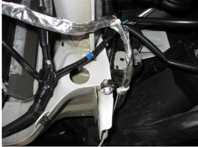
Use a black wire tie to attach the block heater harness to the vehicle wiring harness. Leave approximately one inch of relief in harness to allow for engine movement.
