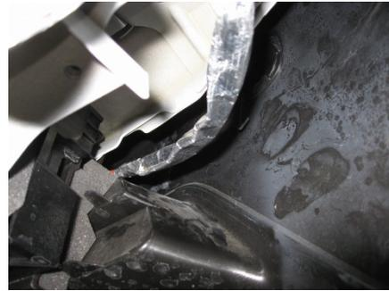
Route block heater harness in front of variable duct and behind vertical support of lower air intake opening.
