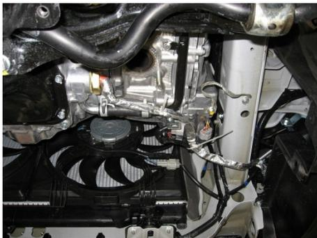
Plug harness into heater element. Orient orange connector towards the front by twisting the orange connector inside the heater. Inside of heater can be rotated relative to the outer body.
