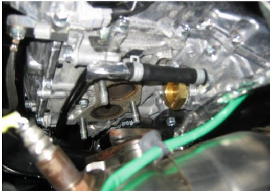
Using the aluminum tape supplied, wrap the CVT transmission coolant line near the point where it attaches to the rubber hose.
