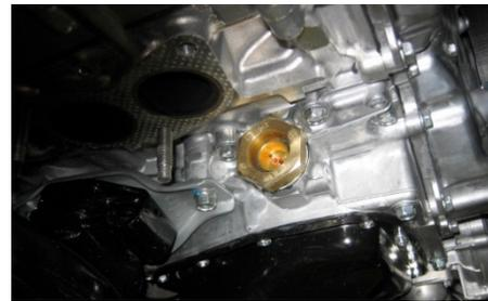
Install engine block heater into core plug opening and tighten with adjustable pliers until gasket is seated completely to engine block. <Reference information> The torque value of block heater plug: 90[N.m] / 66.4 [lb.ft]. **Caution: Failure to follow proper tightening procedures may allow coolant to leak onto the hot exhaust pipe and cause a fire, resulting in serious personal injury and property damage.**
