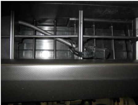
Using the male plug protector strap, attach the male plug to the grill-work in the lower air intake area. **Caution: The harness and the male plug must not interfere with the variable duct.**
