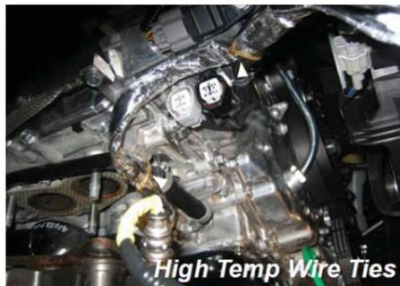
Using the gold high temperature wire tie provided, attach the block heater harness to the taped section of the CVT transmission cooling line. Route the harness forward above the oxygen sensor electrical connectors. Use the second gold high temperature wire tie to attach the block heater harness to the engine harness next to the black oxygen sensor connector.
