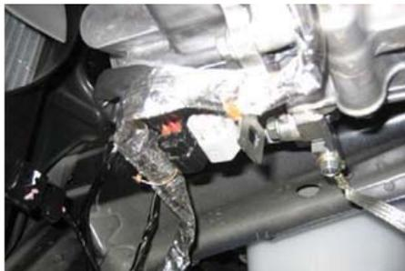
Attach block heater harness to the oxygen sensor bracket and wiring harness using the two high temperature gold wire ties included with the kit.
