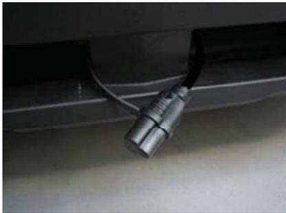
Using male plug protector, attach male plug to grill-work in the lower area.
