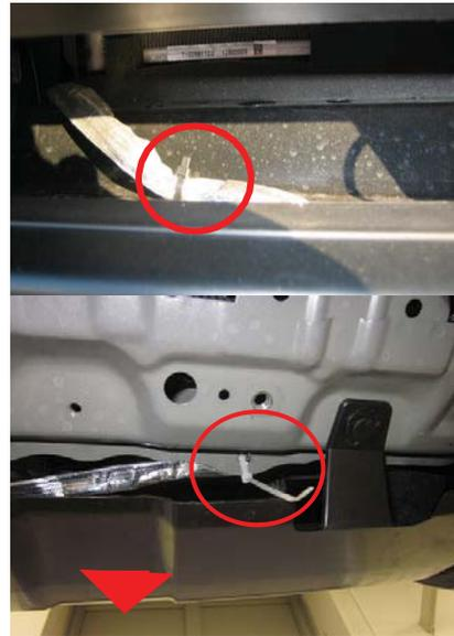
Route harness around the RH side of radiator and condenser towards the front of the car. Using the high strength wire tie loosely attach the harness to the lower radiator support as shown.
