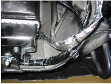
Route harness to the lower right hand side of the radiator. Use the black wire tie to attach the block heater harness to the vehicle wiring harness at the lower right corner of the radiator. Leave approximately one inch of relief in harness to allow for engine movement.
