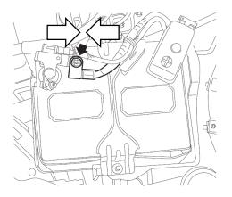
Connect the ground cable from battery.
