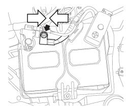
Connect the ground cable from battery.
